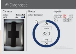
runs through a special verification sequence via CuDDI's software. Using this specially built verification process, an operator can quickly verify the white and black balance of the camera which standardizes the colors, and together with the center square, can verify the measurement or scale reported by the algorithm. CuDDI's software will automatically determine if calibrations are within specifications and prompt the operator when it is time to calibrate, using the same calibration standard.
