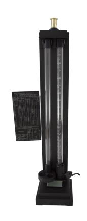
ASTM D156 DIN 51411 SAYBOLT COLOR OF PETROLEUM PRODUCTS (SAYBOLT CHROMOMETER METHOD)
