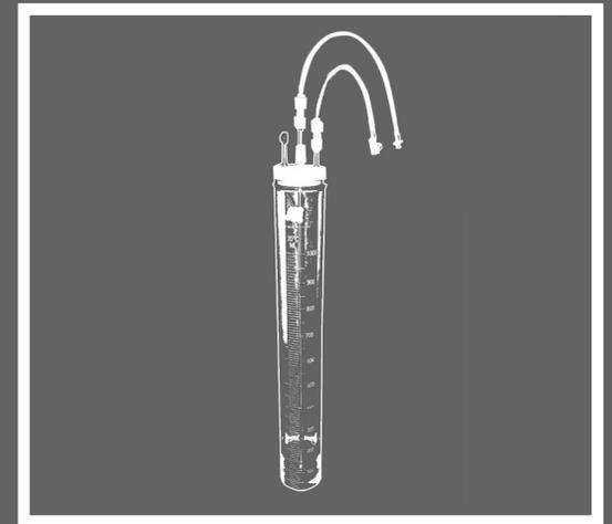
The FOAM Digital Detection Imaging (FoamDDI) apparatus is unique in improving the determination of two of the most important performance parameters of lubricants: The Tendency to foam and the Stability of it. FoamDDI accurately controls the air flow, temperature and sequence, which is then augmented using a unique VISION algorithm to accurately determine the height of static and dynamic foam heights, while greatly improving the precision and accuracy.
